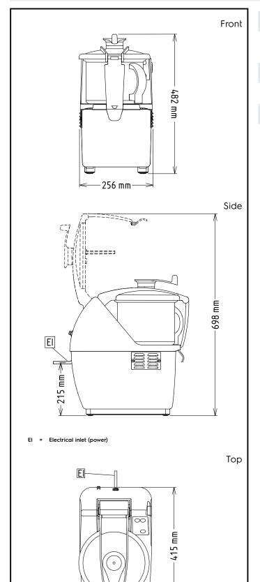
**Electric** Supply voltage: 380-440 V/3 ph/50/60 Hz Electrical power max: 0.9 kW **Total Watts:** 0.9 kW
